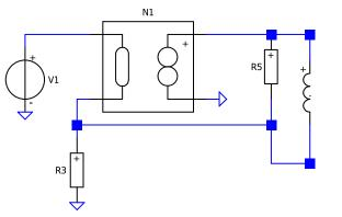
Replace the nullor with the small-signal model of the TLV4111
