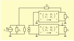
Active feedback Inverting voltage amplifier
