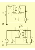
Single-loop passive feedback amplifiers with grounded source and load:
