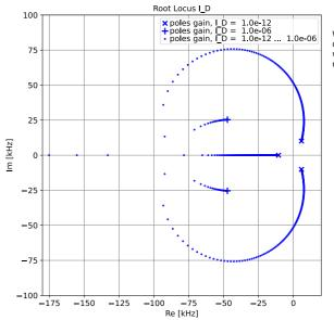
With SLiCAP we can with an arbitrarily selected root locus variable
