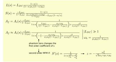
Note: After compensation the servo function itself is not an MFM function because it has a zero. This zero however, is not visible in the gain. Hence, the high-frequency roll-off of the gain with respect to the ideal gain has an MFM characteristic
