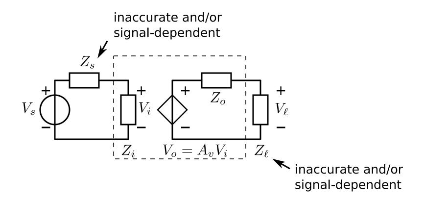
**Brute-force** reduction of the influence of source and load impedance variations on the accuracy of the transfer of a voltage amplifier
