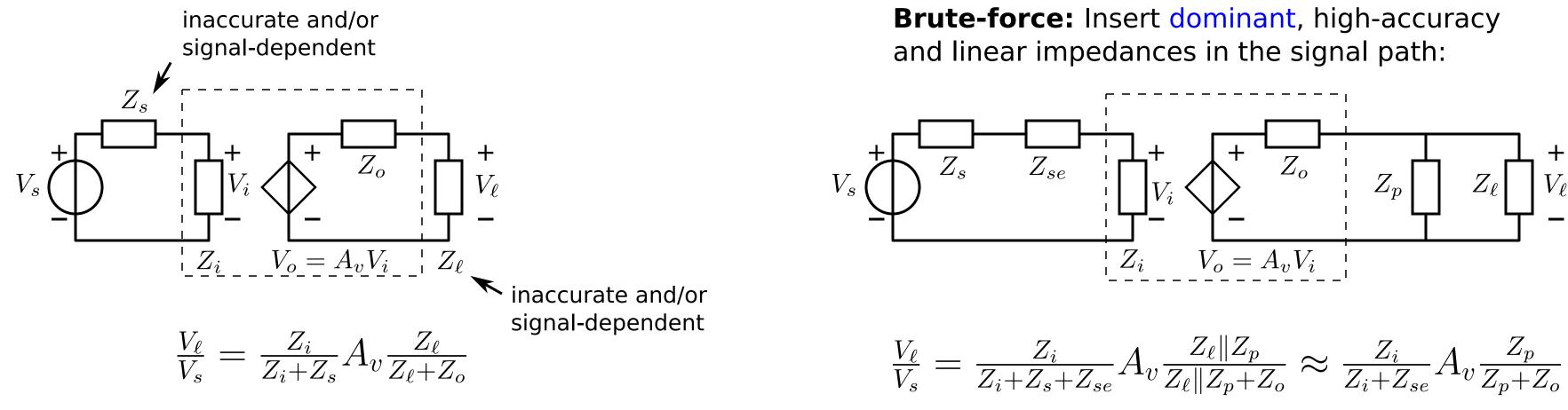
Remember: Thou shalt not insert impedances in U U series or in parallel with the signal path
