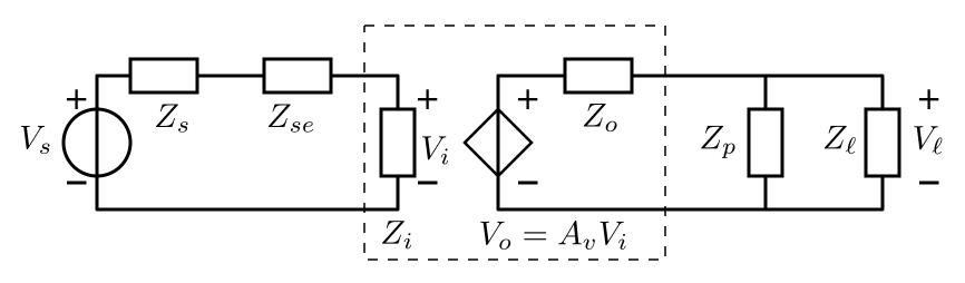
Remember: Thou shalt not insert impedances in series or in parallel with the signal path
