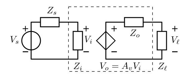
**Brute-force** reduction of the influence of source and load impedance variations on the accuracy of the transfer of a voltage amplifier
