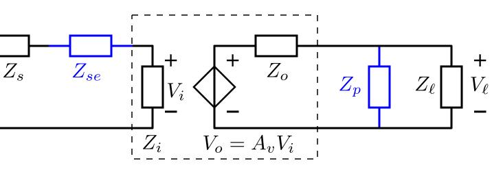
**Brute-force** reduction of the influence of source and load impedance variations on the accuracy of the transfer of a voltage amplifier
