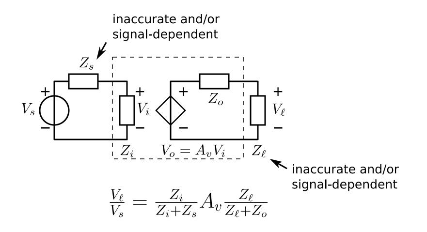
**Brute-force** reduction of the influence of source and load impedance variations on the accuracy of the transfer of a voltage amplifier
