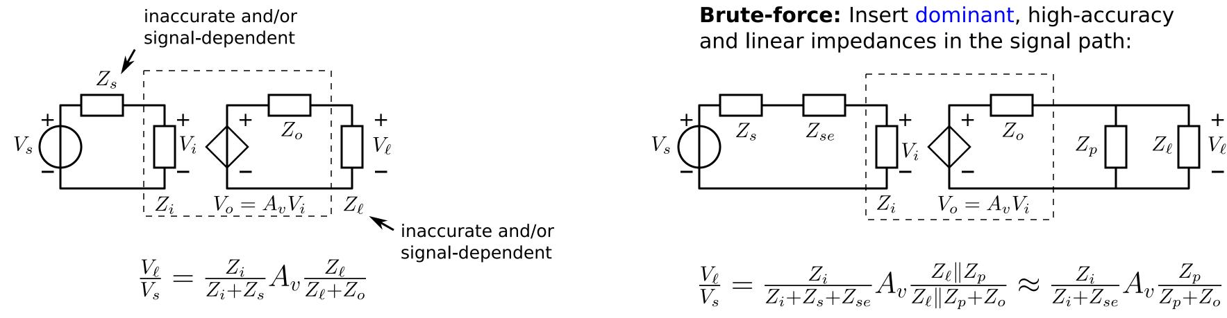
Remember: Thou shalt not insert impedances in series or in parallel with the signal path
