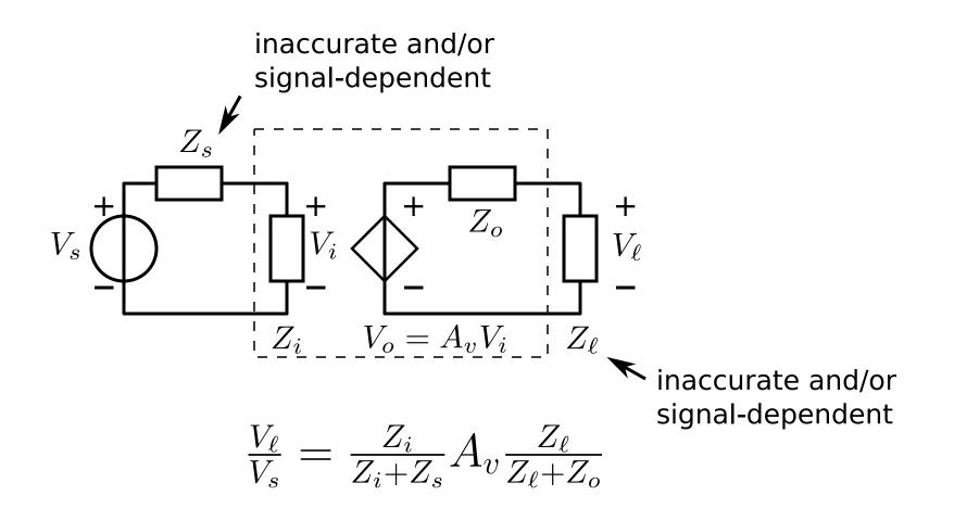
**Brute-force:** Insert dominant, high-accuracy and linear impedances in the signal path:
