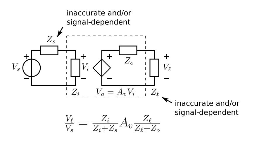
**Brute-force:** Insert dominant, high-accuracy and linear impedances in the signal path:
