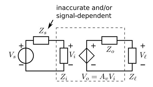
**Brute-force** reduction of the influence of source and load impedance variations on the accuracy of the transfer of a voltage amplifier
