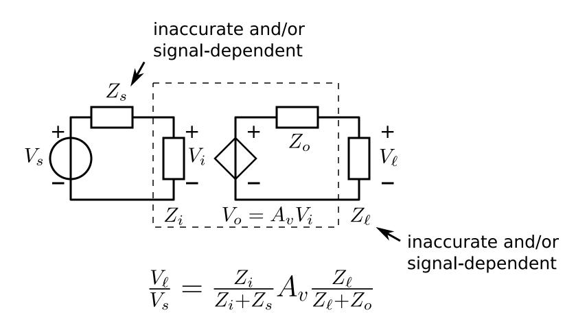
**Brute-force:** Insert dominant, high-accuracy and linear impedances in the signal path:
