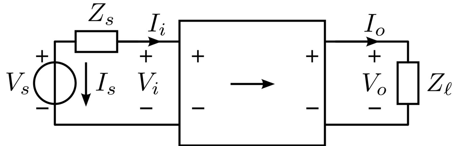
$$\mu = \frac{1}{A} = \frac{V_o}{V_i} \Big|_{I_o=0} \quad A = \lim_{Z_\ell \rightarrow \infty} \left( \frac{V_i}{V_o} \right) \quad \zeta = \frac{1}{C} = \frac{V_o}{I_i} \Big|_{I_o=0} \quad C = \lim_{Z_\ell \rightarrow \infty} \left( \frac{I_i}{V_o} \right)$$
