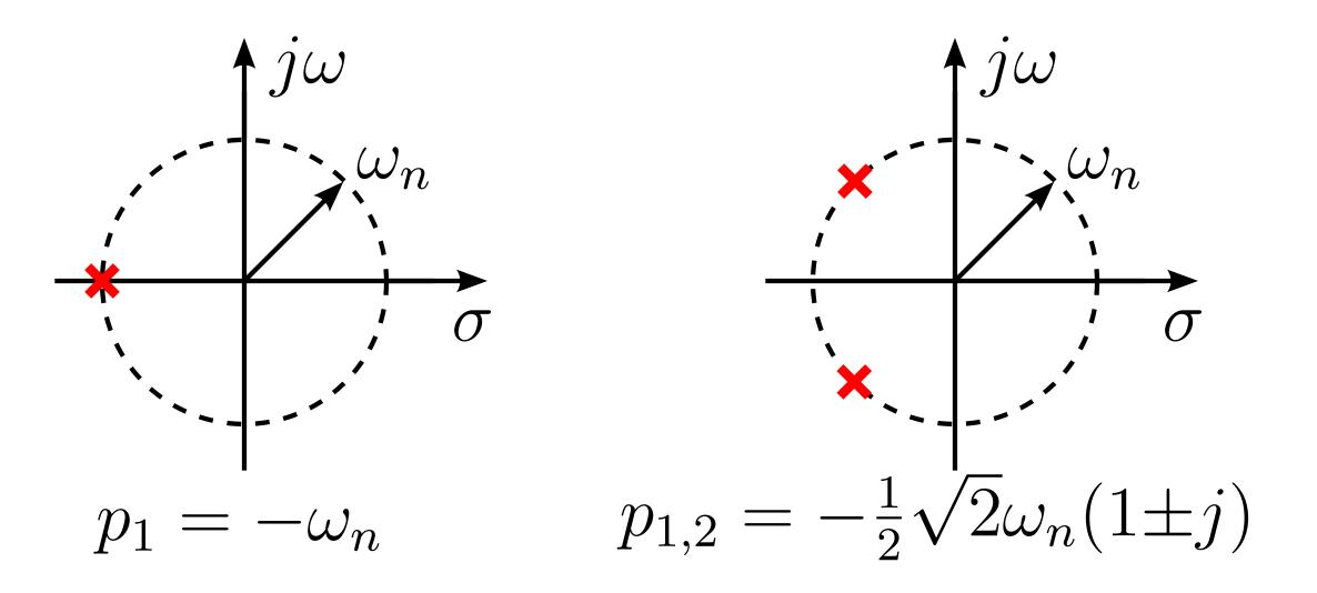
$$H_1(s) = \frac{1}{1+s\frac{1}{\omega_n}} \qquad H_2(s) = \frac{1}{1+s\frac{\sqrt{2}}{\omega_n}+s^2\frac{1}{\omega_n^2}}$$
