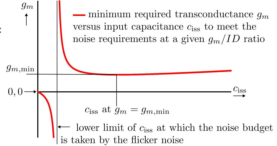
This noise design equation has one minimum transconductance for:  $c_{\rm iss}>rac{lpha}{e_{\ell,s}^2}$
