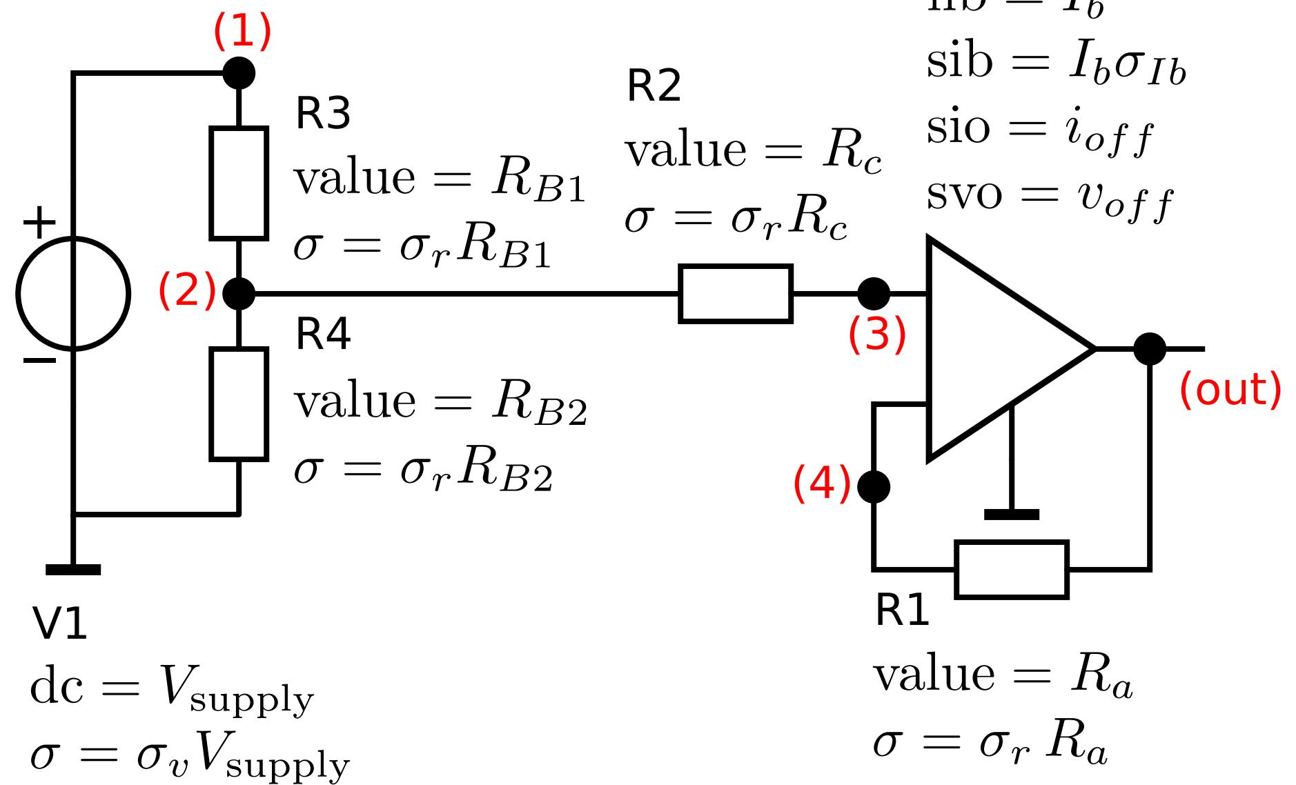
Simplified result:  $R_c \gg \frac{R_{B1}R_{B2}}{R_{B1}+R_{B2}}$
