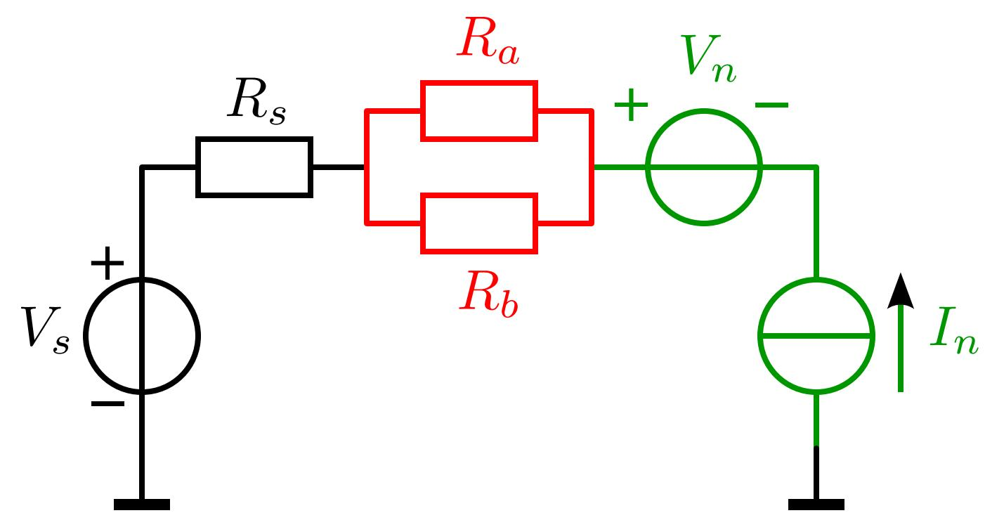
$$S_{v_{tot}} = 4kT(R_s + R_a||R_b) + S_{V_n} + S_{I_n}(R_s + R_a||R_b)^2$$
