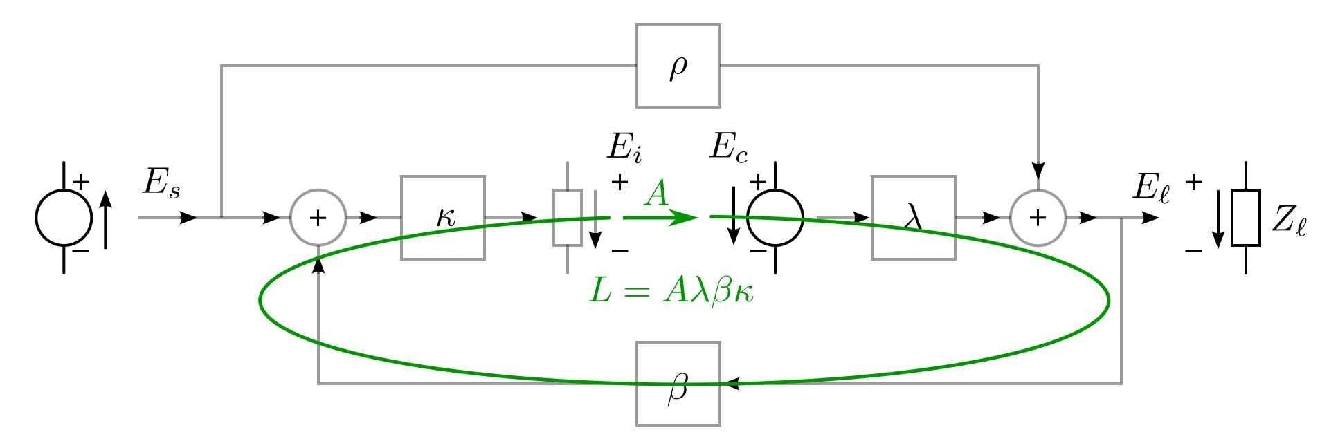
L = Loop gain = gain enclosed in the loop  $= A\lambda\beta\kappa$
