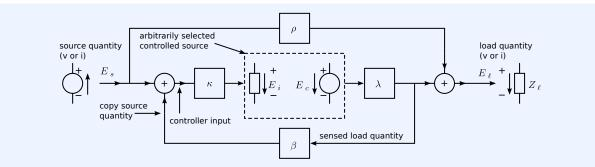
The source-to-load transfer obtained from asymptotic-gain model always equals the source-to-load transfer obtained from network analysis, regardless the selection of the reference variable.
