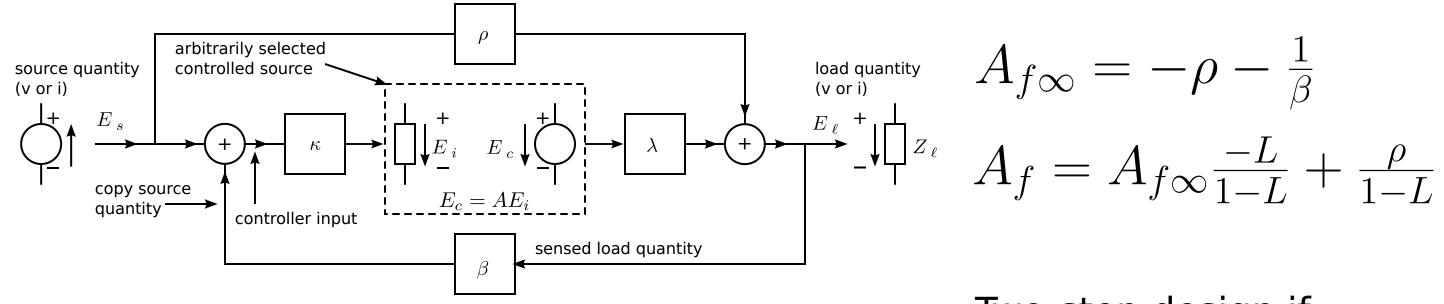
Ideal gain = asymptotic gain if the controller behaves as a nullor in cases in which the gain of the loop gain reference becomes infinity
