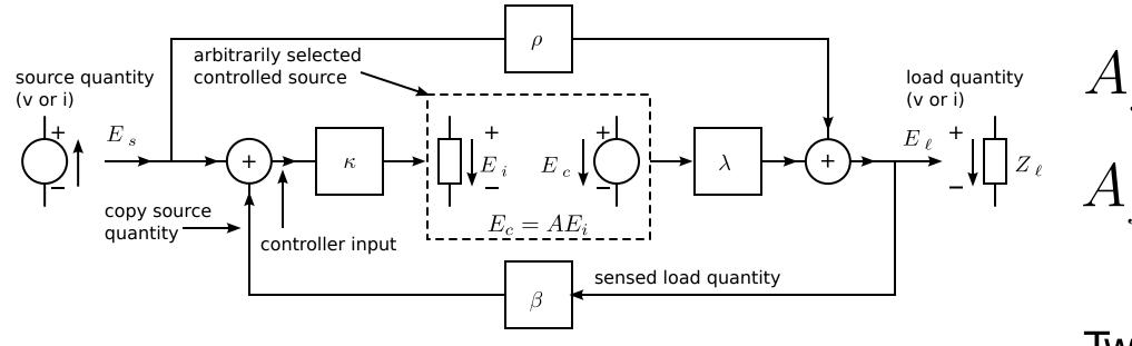
Ideal gain = asymptotic gain if the controller behaves as a nullor in cases in which the gain of the loop gain reference becomes infinity
