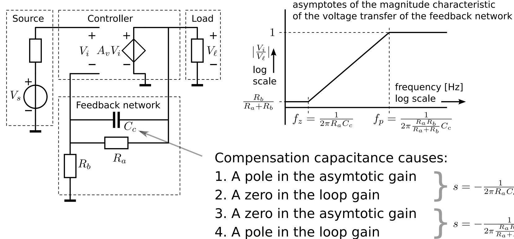
Effective phantom zero (in this case, not a rule!) if:  $R_a \gg R_b$
