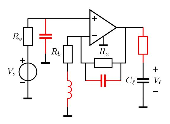
Possible phantom zero implementations in a voltage amplifier with resistive source capacitive load and resistive feedback
