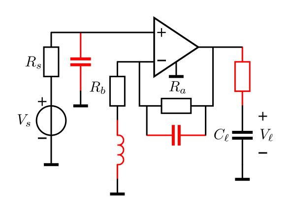
Pole in the asymptotic gain: a. Low-pass transfer from source and input b. Low-pass transfer from output and load c. Zero in feedback network
