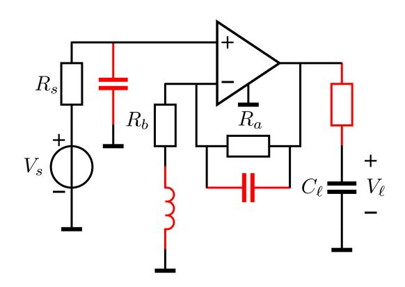
Possible phantom zero implementations in a voltage amplifier with resistive source capacitive load and resistive feedback
